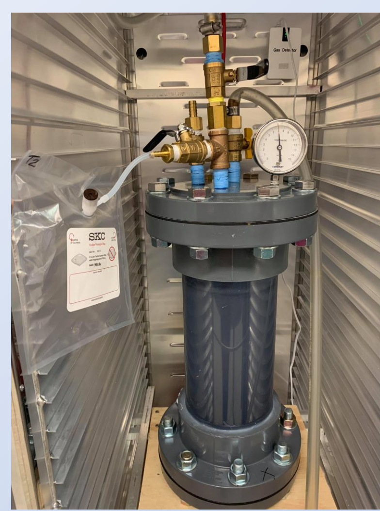
Fig 2. Anaerobic bioreactor attached with Tedlar bags for gas sampling.
