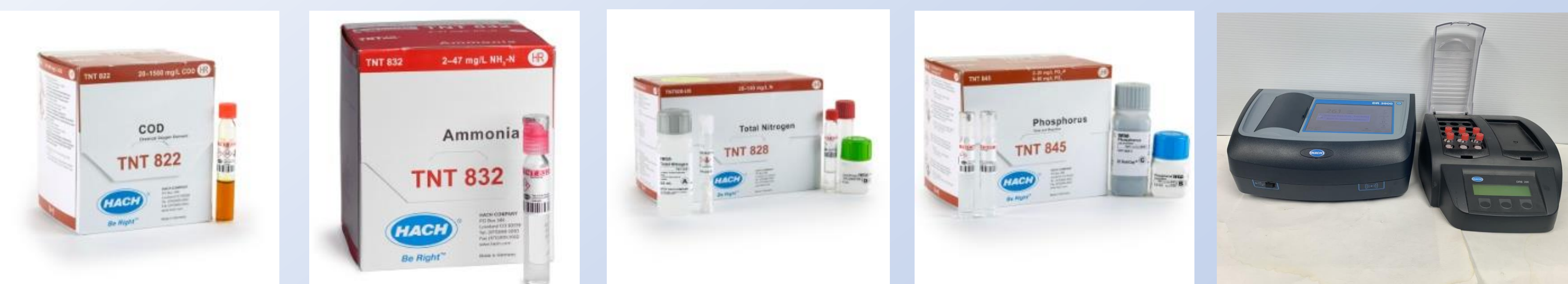
Fig 5. TNT HACH Test kits and spectrophotometer used for analysis of effluent quality.
