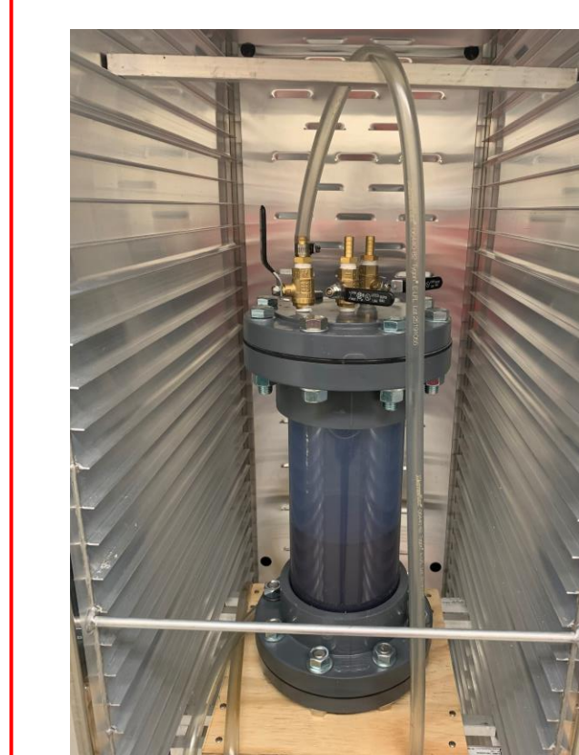
Fig 7.8 . Reactor set up for anaerobic digestion
