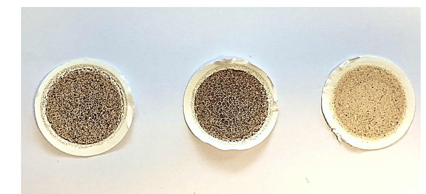
Fig 6. Total Suspended solid on dried filter paper for Control, SS, and SD (left to right).
