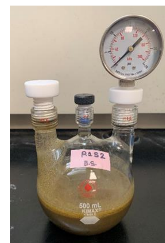
Fig 3. Microcosm set up for batch digestion
