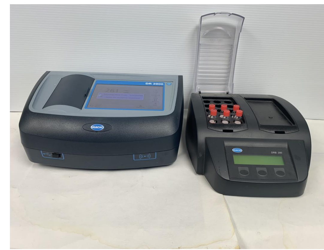
Fig 4. DRB 200 Reactor block and Spectrophotometer for COD analysis of samples
