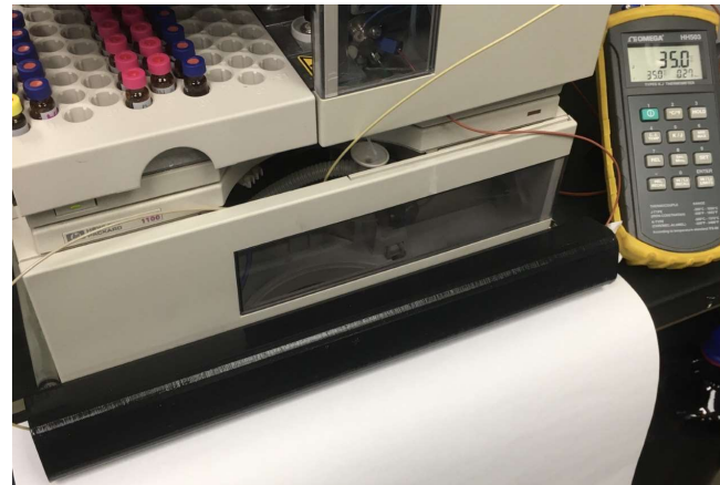
Figure 6: 3D Printed Double Pipe Heat Exchanger Heating HPLC Column
