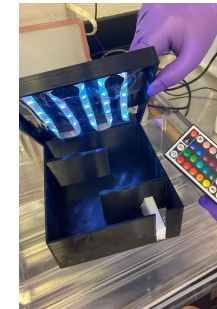
Figure 11: Fully 3D Printed Custom Photo Bio Reactor For Suspended Algae Growth
